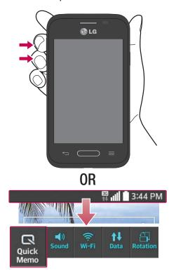
1 Access the **QuickMemo** feature by pressing both Volume Keys for one second on the screen you want to capture.
