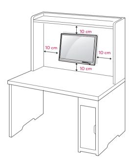
When you install the Monitor set using a wall mounting interface (optional parts), attach it carefully so it will not drop.
