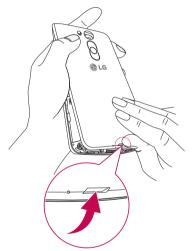
2 Slide the SIM card into its slots as shown in the figure. Make sure the gold contact area on the card is facing downwards.
