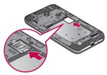
3 Insert the battery into place by aligning the gold contacts on the phone and the battery • and press the battery down until it clicks into place • .
