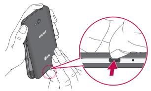
2 Insert the microSD card into the slot. Make sure the gold contact area is facing downwards.
