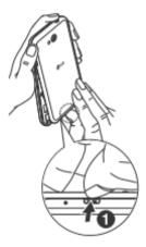
2 Slide the SIM card into its slots as shown in the figure. Make sure the gold contact area on the card is facing downwards.
