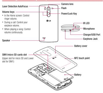
**LDAF Sensor (Laser Detection AutoFocus Sensor):** By detecting the distance with laser, when you recording with the rear camera lens, LDAF Sensor enables you to focus the long or close range more fast and accurately.
