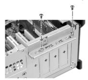
Use the driver and remove the metal slot cover.
