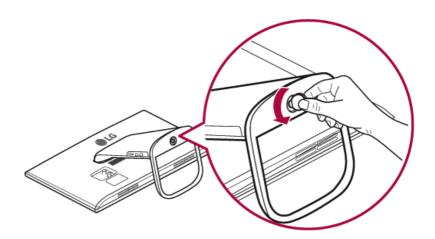
Loosen the two screws at the bottom of the stand using a Philips (+) screwdriver.
