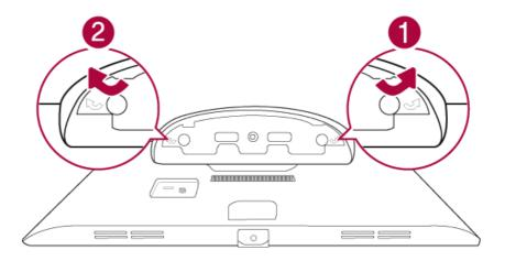
Loosen the two screws indicated in the figure to separate the memory cover.
