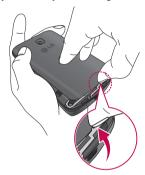
2 Slide the SIM card into slot as shown in the figure. Make sure the gold contact area on the SIM card is facing downwards.
