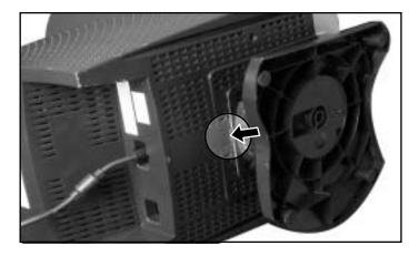
**4** While pressing in the latch, slide the base toward the back of the monitor, then remove the base.
