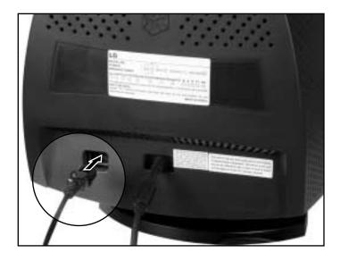
**5** Plug the other end of the power cord into a properly grounded electrical outlet.
