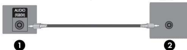
Figure 3-15 Connecting the Audio Cable
