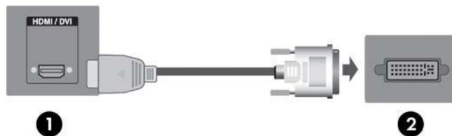
Figure 3-14 Connecting the HDMI to DVI Signal Cable
