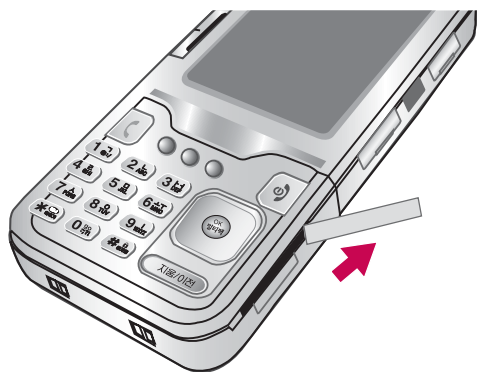
Open the memory card slot
