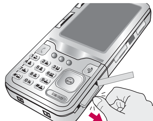
Remove the memory card
