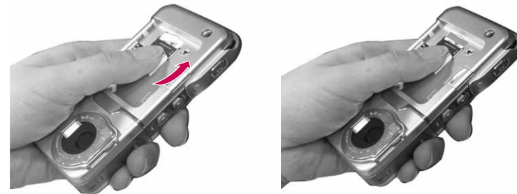
To insert the SIM card
