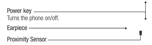
**WARNING:** Moisture on the proximity sensor may cause it to malfunction. Please wipe any moisture off the sensor surface.
