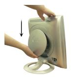
1. Separate the back cap by sliding its lower section downward as shown in the picture.
