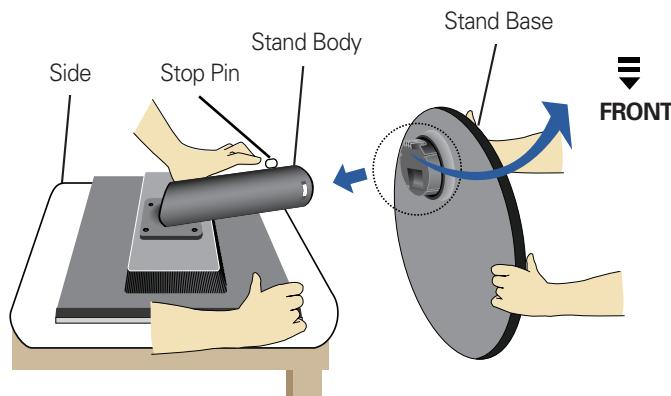
3. Make the monitor stand , then pull out the Stop Pin.
