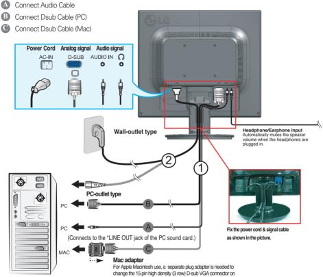
the supplied cable to a 15 pin 2 row connector.
