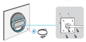
Kensington Security Slot- optional Connected to a locking cable that can be purchased separately at most computer stores **VESA** wall mounting
