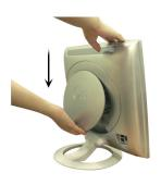
1. Separate the back cap by sliding its lower section downward as shown in the picture.
