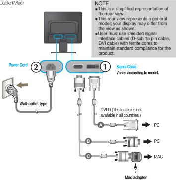
For Apple Macintosh use, a separate plug adapter is needed to change the 15 pin high density (3 row) D-sub VGA connector on the supplied cable to a 15 pin 2 row
