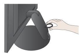
2. After connecting the cables neatly, arrange the cables to the Cable Holder as shown in the following figure.
