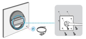
Kensington Security Slot- optional Connected to a locking cable that can be purchased separately at most computer stores **VESA** wall mounting
