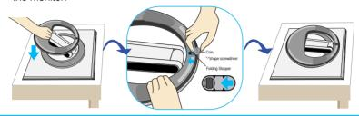
■ Tighten the four **5** screws about half into the slots in the base part, hold the two screws at the bottom to pull them inward, and then tighten the screws all the way.
