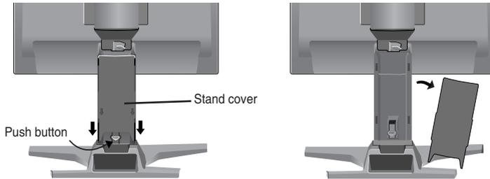
2. After connecting cables, put the **stand cover** correctly into the holes on the stand. If securely connected, you can hear the click sound from the latch.
