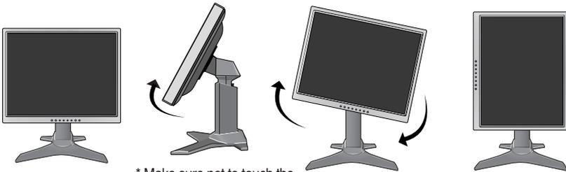
\* Make sure not to touch the floor when the head rotates to use the Pivot function.
