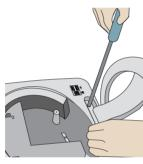
**3.** Separate the stand base using a screwdriver as shown in the picture.
