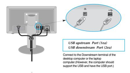
${f 3.}$  The monitor's USB Display terminal supports USB 2.0 and High Speed cables.
