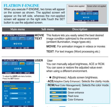
Select the **SAVE** sub-menu using the **SET button** and save the **YES** value using the **buttons**.
