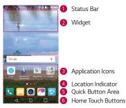
**1** Status Bar - Shows the device's status information, including the time, signal strength, battery status and notification icons.
