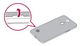
2 Insert the memory card into the memory card slot.
