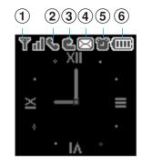
(1) T 1 ~ T : Shows the level of the received radio waves
