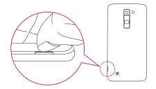
2 Slide the SIM card into the SIM card slot as shown in the figure. Make sure the gold contact area on the card is facing downward.
