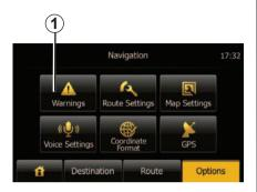
The "Navigation Settings" menu allows you to change the display of the map or navigation parameters.
