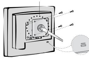
Kensington Security Slot- optional Connected to a locking cable that can be purchased separately at most computer stores
