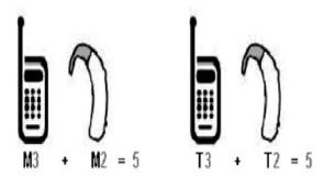
In the above example, if a hearing aid meets the M2 level rating and the wireless phone meets the M3 level rating, the sum of the two values equal M5. This is synonymous for T ratings. This should provide the hearing aid user with "normal usage" while using their hearing aid with the particular wireless phone. "Normal usage" in this context is defined as a signal quality that is acceptable for normal operation.
