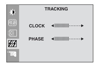
Clock. Press the < and > buttons to minimize any vertical bars or stripes visible on the screen background. The horizontal screen size will also change.
