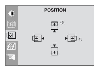
**Vertical position.** Press the  $\triangle$ and  $\nabla$  buttons to move the image up and down.
