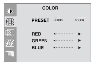
**Preset.** Press the ⊲ and ⊳ buttons to adjust the color temperature. 9300K is bluish white. 6500K is reddish white.
