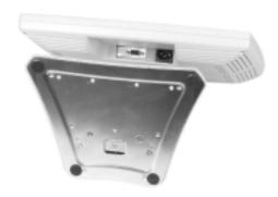
4 Connect one end of the video cable to the matching video port on the underside of the display.
