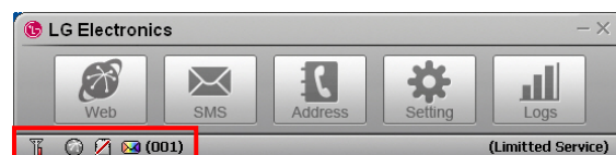
When LHU2100T is connected but USIM Card is not inserted or is improperly inserted
