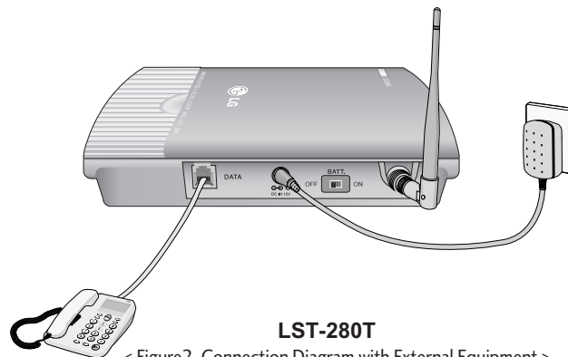
< Figure2. Connection Diagram with External Equipment >
