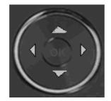
As you navigate through a menu, the options are highlighted (Highlighted Test Example). Select an option by highlighting it and pressing **OK**. The scroll bar at the right of the menu keeps track of your position in the menu at all times.
