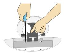
2. Separate the stand base using a screwdriver as shown in the picture.
