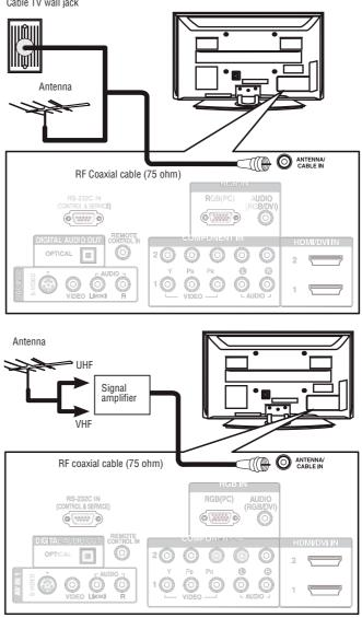
To connect an external antenna, cable TV, or satellite TV:
