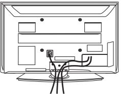
2 Install the cable management clip to route the cables. If your TV has cable holders, install them to bundle the cables.
