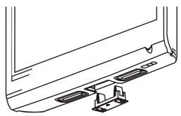
**3** Mount the wall bracket to the TV, using the screw holes indicated in the illustration.
