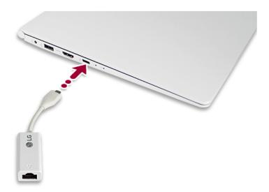
2 Connect the wired LAN cable to the LAN port.
