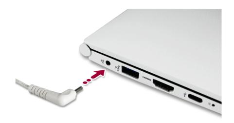
2 Open the LCD and check the charging state. When the AC adapter lamp is blinking, charge it fully with the AC adapter before using it.
