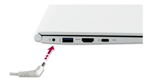
2 Open the LCD and check the charging state. When the AC adapter lamp is blinking, charge it fully with the AC adapter before using it.
