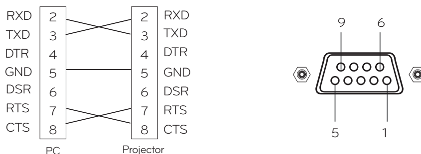
[Figure 1] RS-232 Connection Diagram
