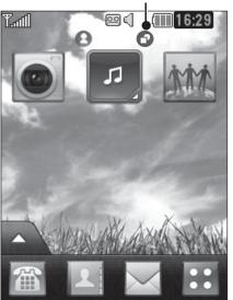
Widget home screen - When you touch on the bottom left of the screen, the mobile widget panel appears. When you register widget by dragging it, the widget is created in the spot.
