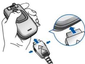
1. With the arrow facing you as shown in the diagram push the plug on the battery adapter into the socket on the bottom of the phone until it clicks into place.
