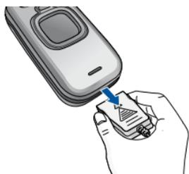
Disconnect the travel adapter from the phone by pressing its side buttons as shown in the diagram.
