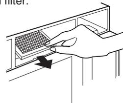
6. Slide a new charcoal filter into place and close the door. The filter should rest at the angle shown.
