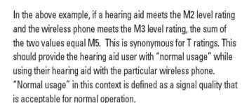
The M mark is intended to be synonymous with the U mark. The T mark is intended to be synonymous with the UT mark. The M and T marks are recommended by the Alliance for Telecommunications Industries Solutions (ATIS). The U and UT marks are referenced in Section 20.19 of the FCC Rules. The HAC rating and measurement procedure are described in the American National Standards Institute (ANSI) C63.19 standard.
