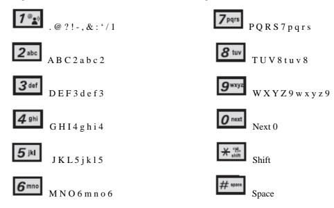
After a character is entered, the cursor automatically advances to the next space after one seconds. You can also advance the cursor by pressing "Right Navigation Key" or entering a character not on the same key.
