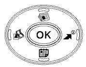
As you navigate through a menu, the options are highlighted (Highlighted Test Example). Select an option by highlighting it and pressing OK. The scroll bar at the right of the menu keeps track of your position in the menu at all times.
