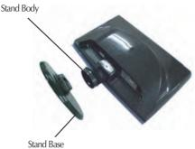
**3.** Tie down the base lock to perpendicularity direction.
