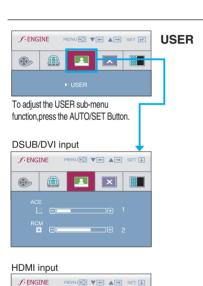
You can manually adjust brightness, **ACE** or **RCM** (only for DSUB/DVI input), **HUE** or **SATURATION** (only for HDMI input).
